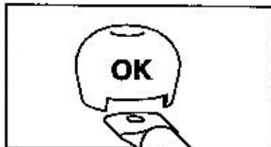
Field distributor positioned correctly
